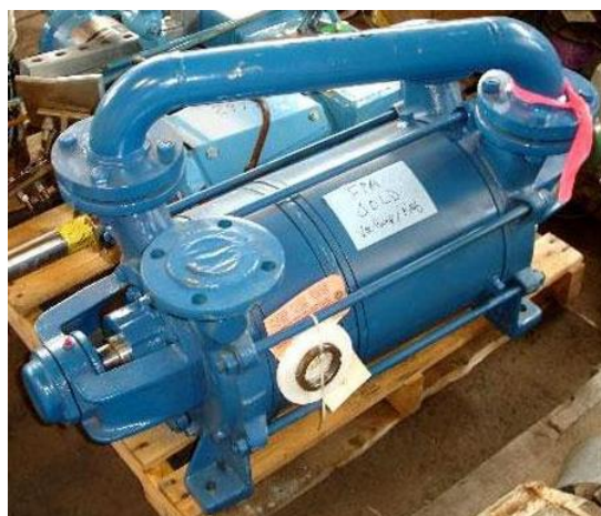
Gambar 6. Pompa vakum liquid ring two stage di lokasi penelitian
